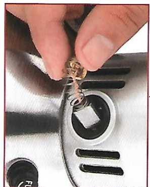
As for the replacement of the carbon, screw tightly as the above sketch shows
